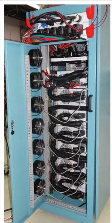
Rear View with Door Open showing Cable Arms for Each Pull-Out Box 6 Unit Test Cables from Chamber to System
