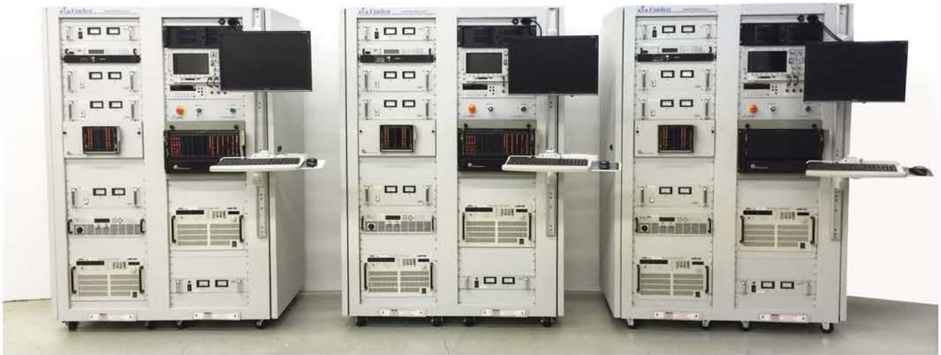
Three Duplicate Testers for Production Test
