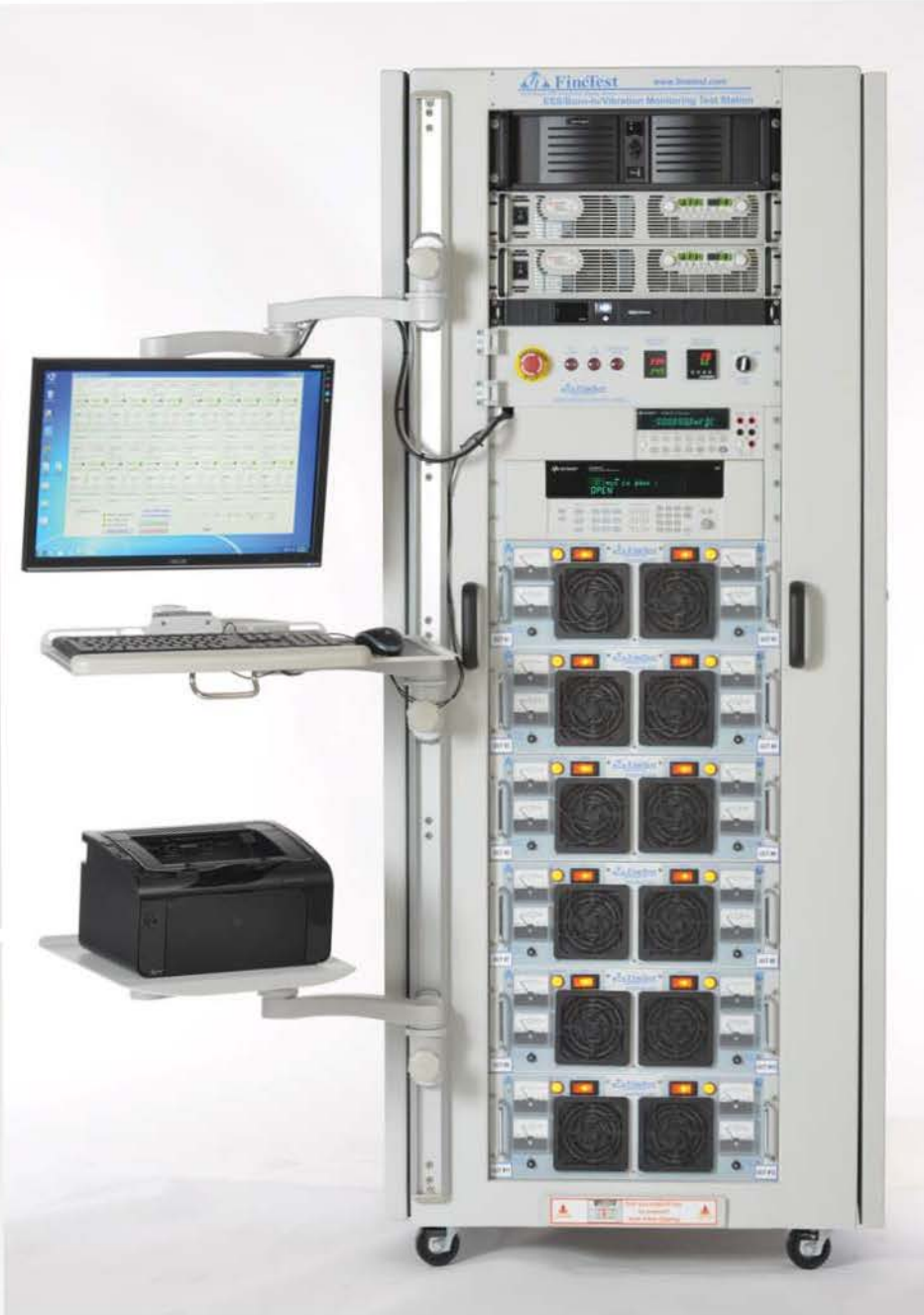
Front view of ESS, Burn-In and Vibration Monitoring System
