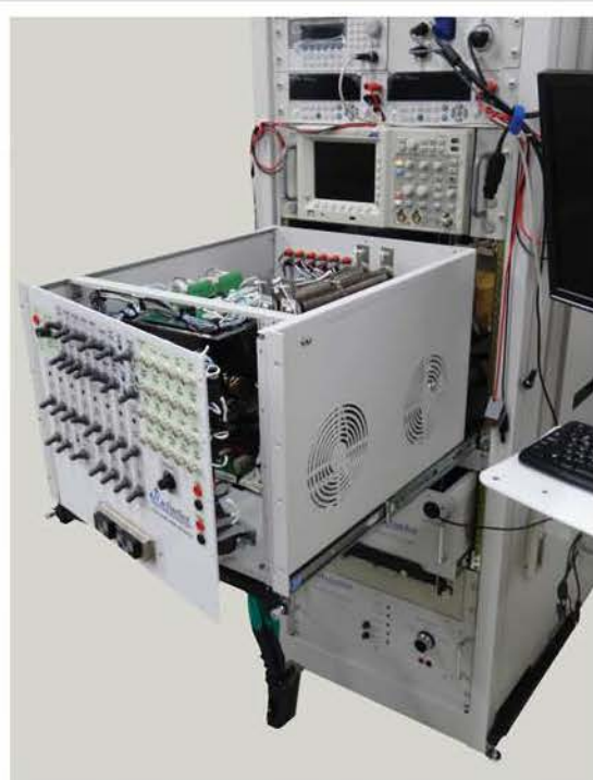
Interface Unit is on Slide-Out Shelf, with removable Top and Front Door
