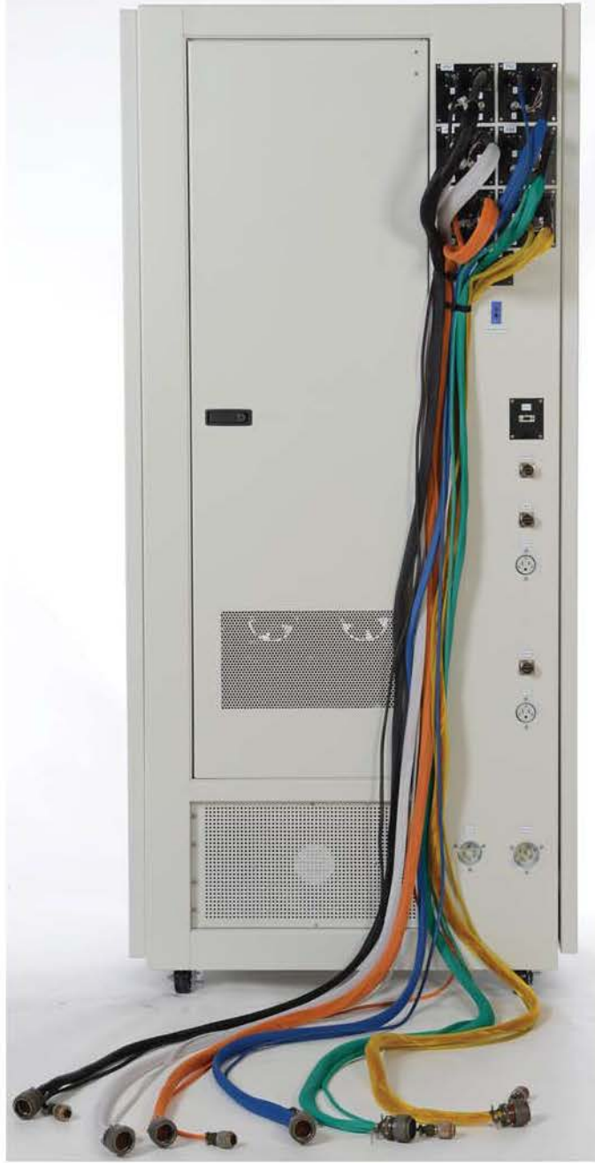
Rear view of System showing Color-Coded Temperature Rated Cables that connect the System to the UUTs inside the Thermal Chamber
