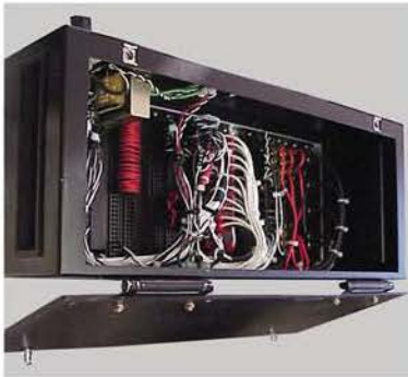
Self-Test ITA with cover open to show wiring
